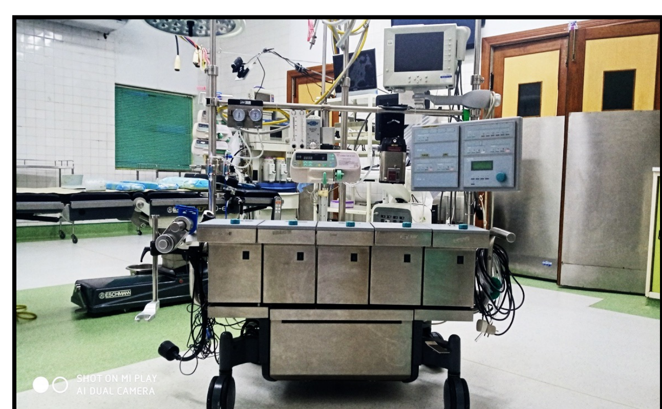
Stockert S III Heart lung machine with Terumo CDI-550 blood parameter inline monitor
